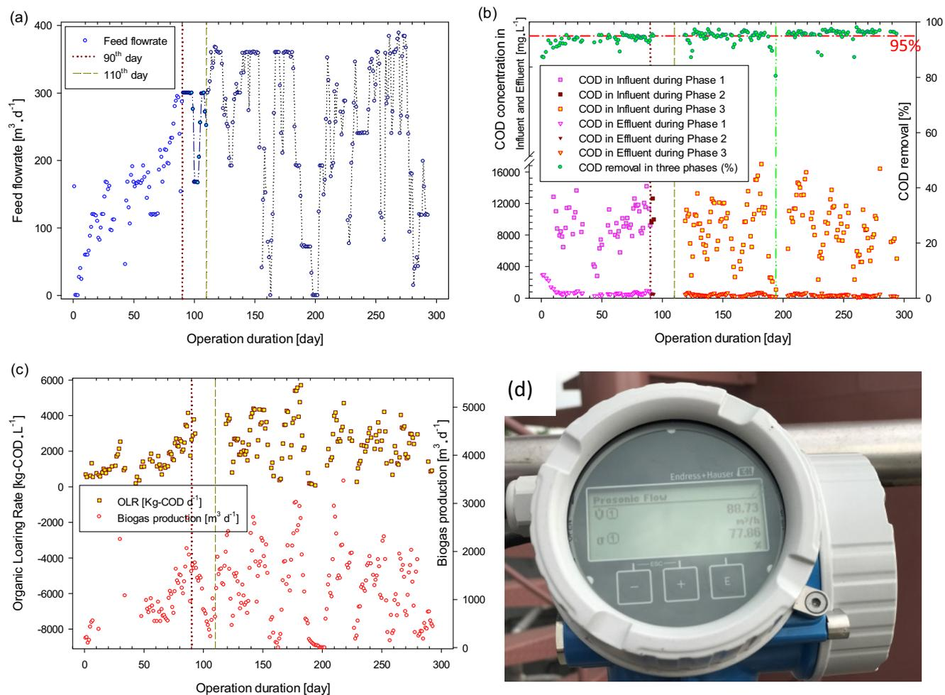
**Fig. 3** **a** Feed flow rates in three phases (separated by dotted and dashed lines on 90th and 110th day, respectively); **b** COD in the influent, effluent, and removal; **c** OLRs and biogas production rates; **d** biogas monitoring transmitter
