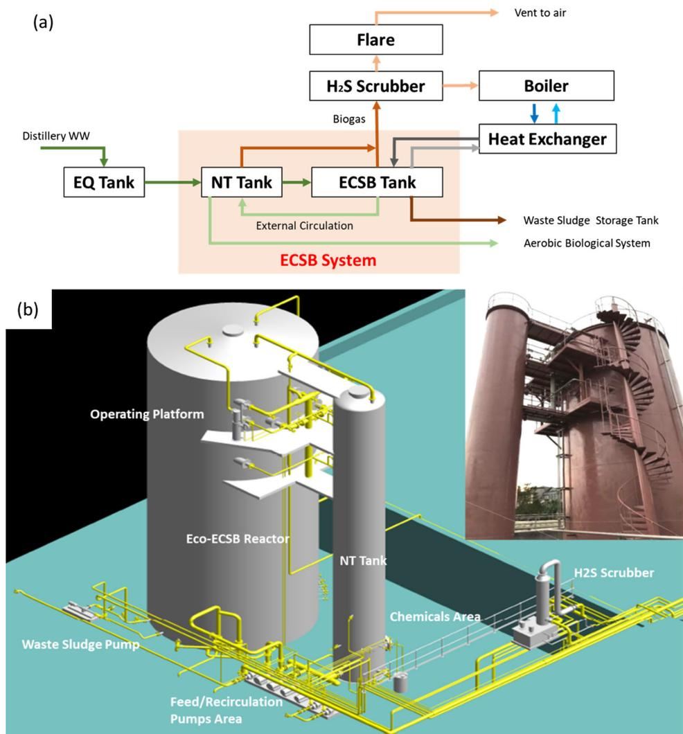
supernatant from the anaerobic system flowed into the aerobic biological system. Patent design of gas collection piping system in the ECO-ECSB™ can check fouling under the G-L-S separator during operation. In case fouling occurred, it is also capable to clean the separator directly either by the biogas or from the external water pipes. Therefore, the system can continuously run without intensively scheduled checks or maintenance.
