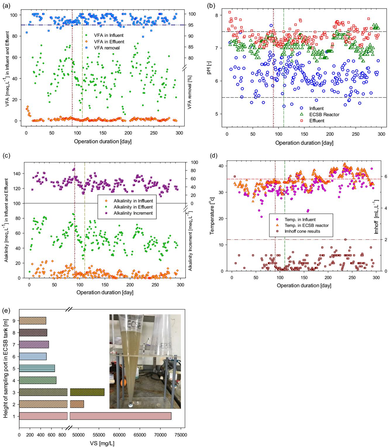
**Fig. 4** a VFA in the influent, effluent, and removal; b pH in the influent, ECSB tank, and effluent; c alkalinity in the influent, effluent, and increment; d temperatures in the influent and ECSB tank; e VS of sludge from nine sampling ports and the Imhoff cone test apparatus
